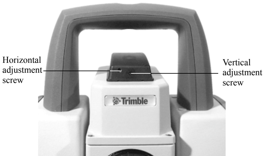
Figure 8.2 Laser Pointer adjustment screws
