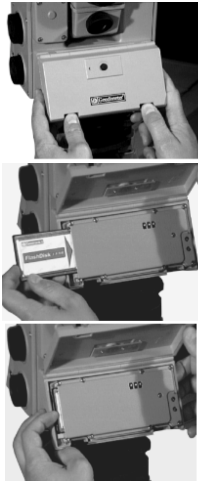
Figure 12.5 How to insert the memory card into the card memory device.
