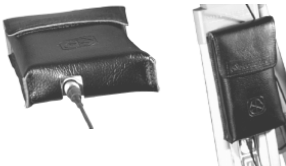
Figure 12.2 How to connect the card memory using the system cable.
