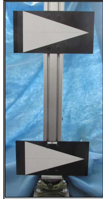
Figure 4-24. - Example of recommended target assembly.
