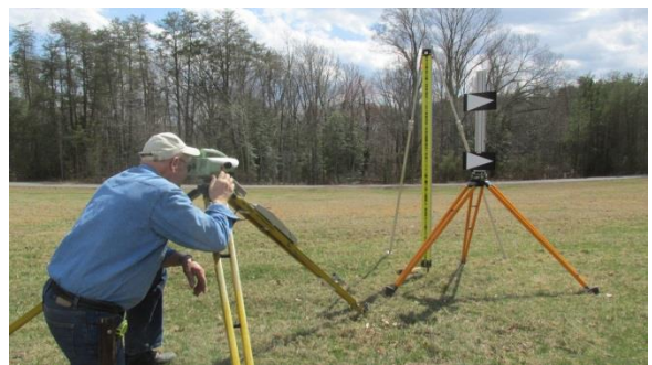
Figure D-2. Sighting on the lower target triangle point.
