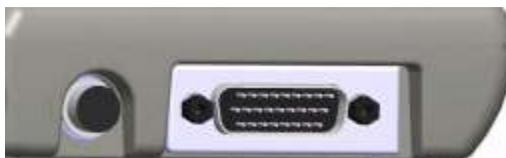
Figure 3.3 ACU serial and Hirose ports
