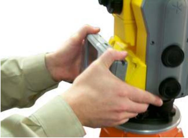
Figure 3.2 Attaching the ACU
