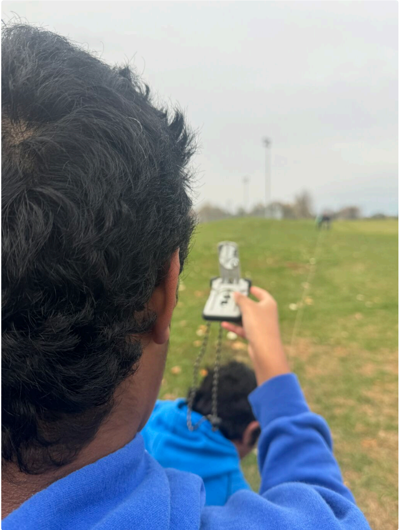
A student uses a compass and string to resurvey an imaginary township that is missing a corner monument.
